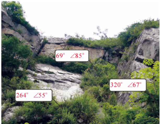
图 4 物源区基岩节理产状 Fig.4 Rock mass joint attitude in provenance
