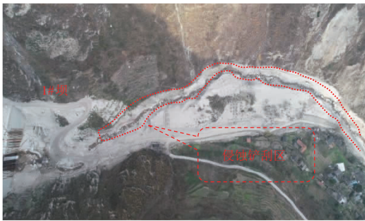
图 7 1#拦砂坝下游沟道铲刮侵蚀(8.20 后) Fig. 7 Spade erosion of gully downstream of No. 1 dam (after August 20)
