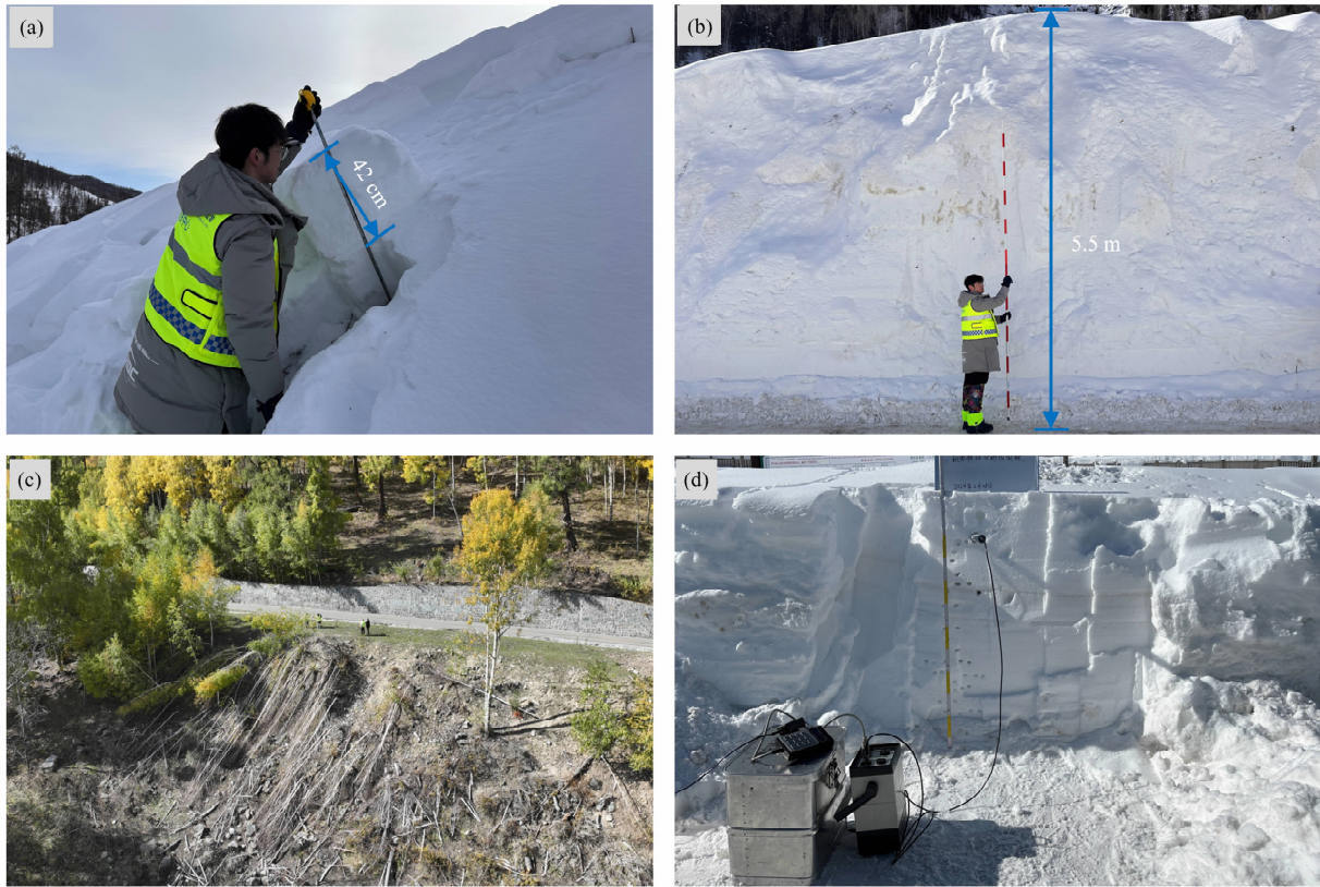
图2 喀纳斯山区雪崩灾害野外勘探调查:(a)雪崩断裂深度;(b)堆积体高度;(c)雪崩损毁树木;(d)雪特性分析 Fig.2 Field investigation in the Kanas region: (a) avalanche fracture depth; (b) deposit height; (c) avalanche-damaged trees; (d) snow characteristics survey
