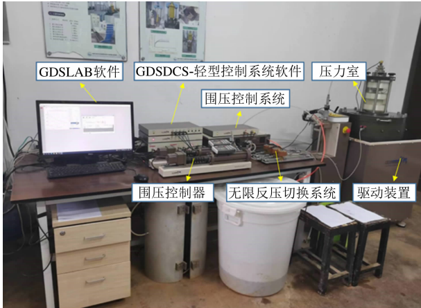
图 3 GDS-DYNTTS 型微机控制三轴试验系统 Fig. 3 GDS-DYNTTS microcomputer-controlled dynamic triaxial test system
